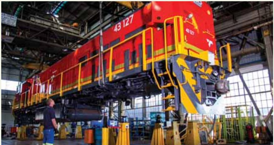
Koedoespoort Bay 1: Vincent Coetzee (engine/alternator alignment) moving new Class 43 locomotive into position.
