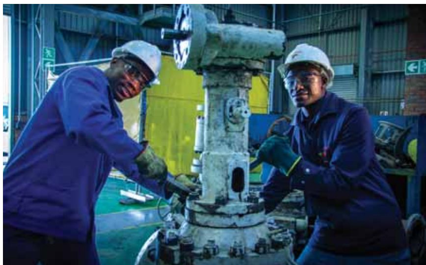
Alrode workshop: Samuel Mokoena (Mechanical artisan) and Sifiso Nkosi (Trade assistant) assembling a four way valve.
