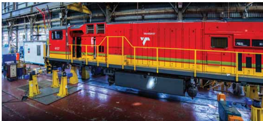
Koedoespoort Bay 1: New Class 43 diesel locomotive under construction.
